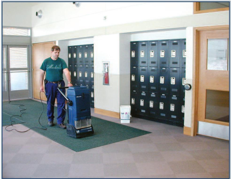
*The HOST Liberator features a dual-brushing action which excels at vacuuming the 6 ft. x 20 ft. ribbed, walk-off mats that trap much of the sand and soil tracked in at the library's two entryways.*
