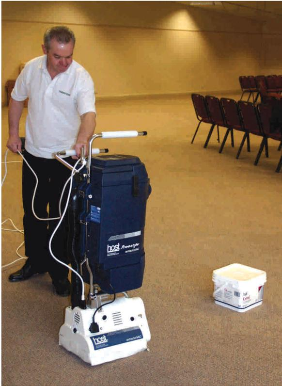
The powerful **ExtractorVac vacuum** removes the dry soil that is freed by this brushing action, even right down to the carpet backing. This is a critical step, given that up to 85% of the soil in carpet is dry and can be removed by this unique system.
