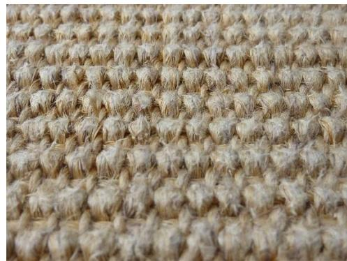
Damage caused by brushing across raised loops and incorrect (too harsh) brush selection
